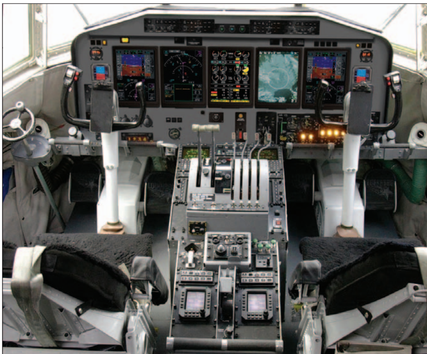
Five-panel display system included in the ASB Avionics L-382/C-130 AMP solution.
